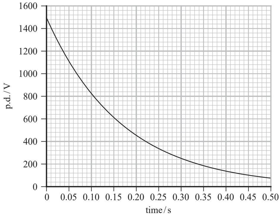
(a) Describe how a graph of p.d. against time can be used to show that the racquet contained a capacitor. Your answer should not include calculations.
