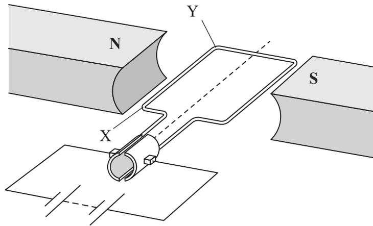
The current in the coil is 0.4A. The magnetic flux density is 0.07T. The length of XY is 5 cm.
