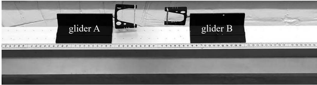
Glider A had mass  $m_A = 0.50 \text{ kg}$  and moved towards glider B at a speed of  $0.60 \text{ ms}^{-1}$ . Glider B was initially at rest.
