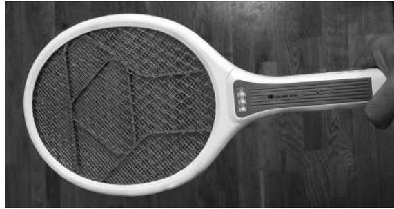
The racquet has two metal meshes. When a fly is between the meshes, the user presses a button and a potential difference (p.d.) of 1500 V is applied between the meshes for a short time. This p.d. causes a current in the fly, stunning it.
