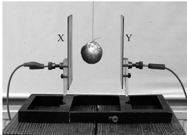
A ball coated in conducting material is suspended, on a very long insulating thread, between metal plates.
